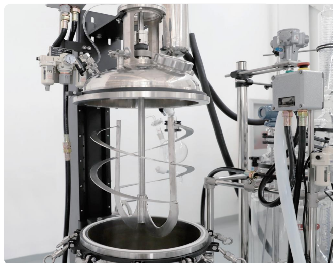
Jacketed Reactor with Ribbon Spiral Belt Impeller
